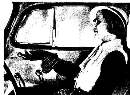
Fig. 12. The front ventilators are operated by the smaller of the two cranks.
